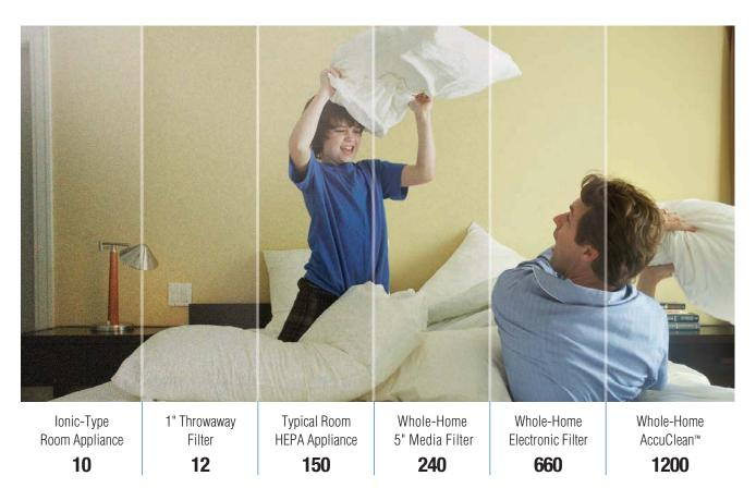
Ratings of cubic feet per minute of clean air delivered for a typical 3-ton heating and cooling system: the higher the value, the more effective the air cleaner. Clean air delivery rate (efficiency times airflow rate) is recognized by the Federal Trade Commission (FTC) and Environmental Protection Agency (EPA) as a fair and objective measure of various air cleaner technologies.
